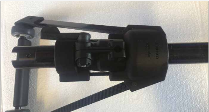
Step 5: Slide magnet roller and collar back onto the tube section.
